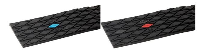
Thickness variation (all strips/pulley) +/-0.5mm. Product code for different lengths: Add 5 digits indicating the overall strip length in mm. Strip length to always be 100mm longer than face width to allow overhang for trimming after application.
